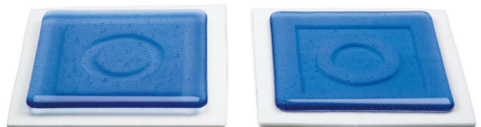
Figure 3b: Fiber paper designs stacked with 6 mm pre-fused glass, before kilncarving firing.
