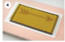
Arrange the fiber paper on a primed kilnshelf. Clean the billet and load it on the fiber paper. Fire with the schedule below.
