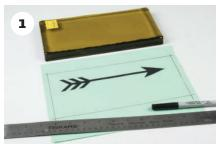
Plan a design based on the billet dimensions, approximately  $10^{\circ} \times 5^{\circ} \times 0.75^{\circ}$  (127 × 254 × 19 mm).
