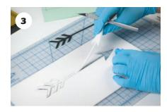
Trace the design onto 1/8" Fiber Paper (7036) and cut it out using an X-Acto knife. For a raised design, oversize the fiber paper by 0.5" on each side to keep the billet from flowing over the edge.
