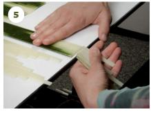
Run your score lines. You can run multiple strips at once by sliding a section to the edge of the table and using the table to snap the score lines.
