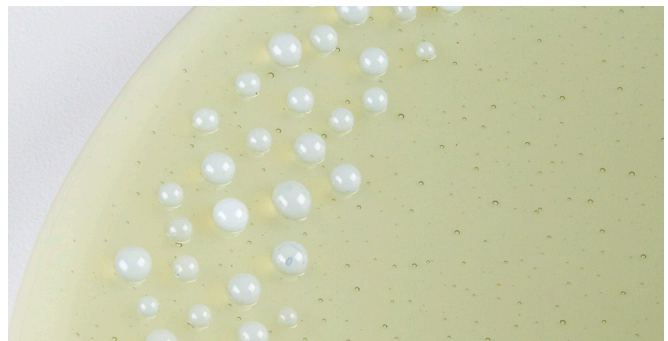
Frit balls made with Opaline Striker coarse frit (000403-0003). (Top and middle) Tack fused together, then slumped. (Bottom) Tack fused to a fully fused plate, then slumped.
