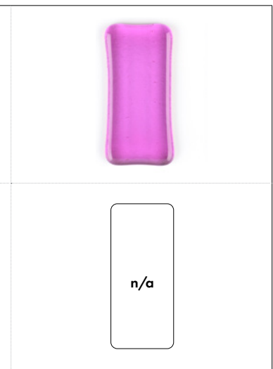
FIRED RESULTS-TEST 2 RUBY PINK TINT 001831-0030 1200°F/648°C | 2 HOUR HOLD
