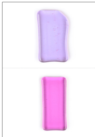
FIRED RESULTS-TEST 1 RUBY PINK TINT 001831-0030 1225°F/663°C | 2 HOUR HOLD
